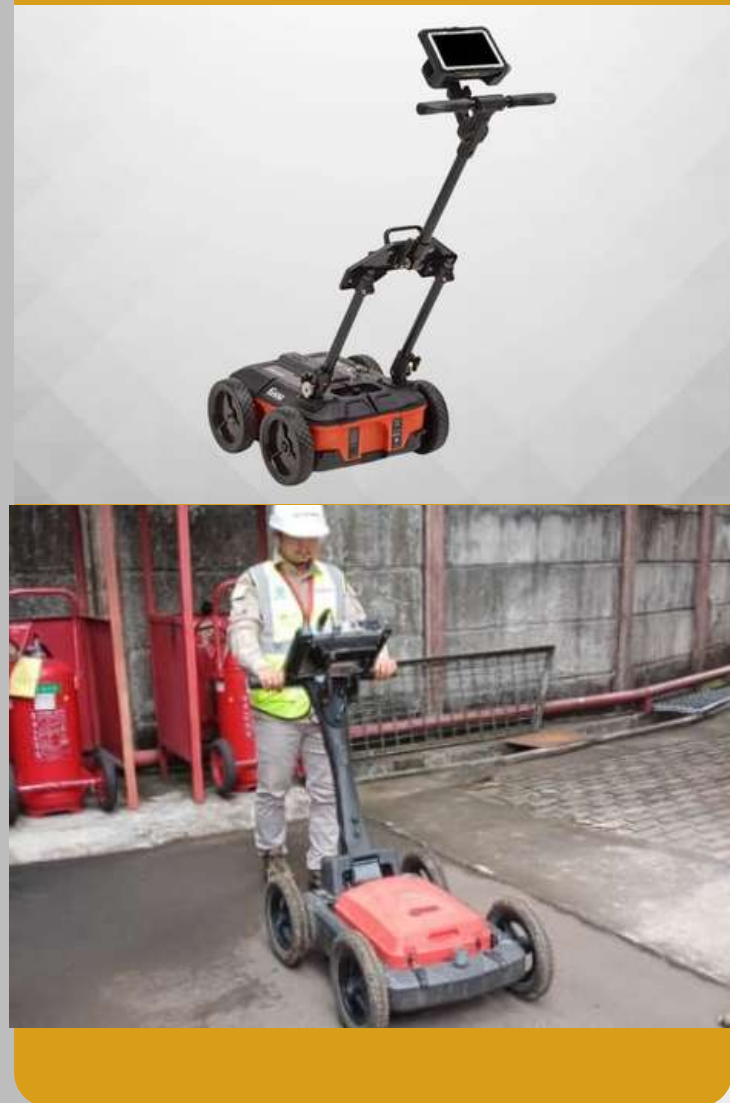
Geo Penetrating Radar
