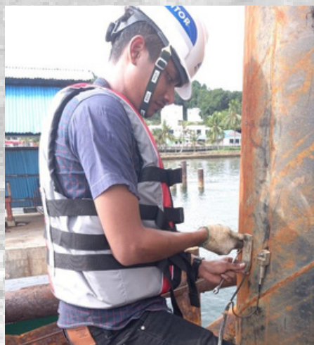
Project PDA Test Struktur Jetty di Terminal BBM - Sorong Papua
