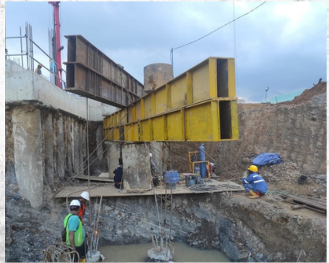
Project JASA UJI PONDASI (PDA, PIT, CSL, Static Axial Load Test) KANTOR INSTANA PRESIDEN IKN
