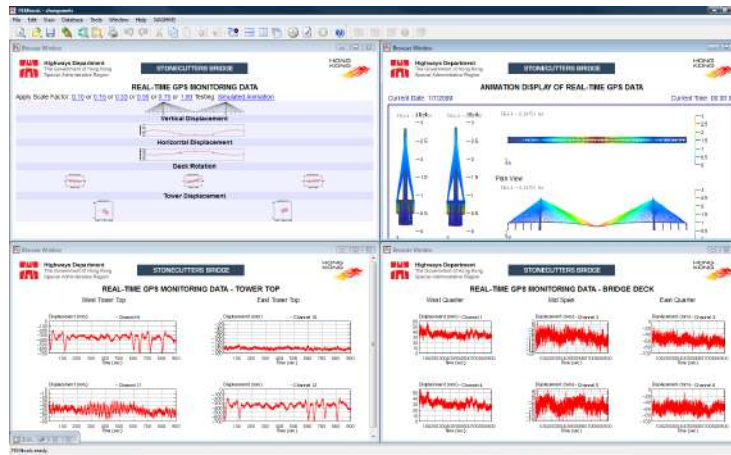
Displacement Monitoring (4-in-1 Display)
