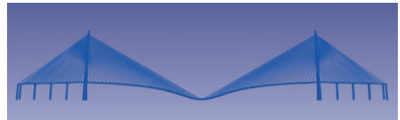
Deformed FE model based on expanded test GPS data
