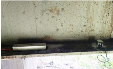
Structural Health Monitoring System (SHMS) Jembatan Lematang - PT Mustika Indah Permai
