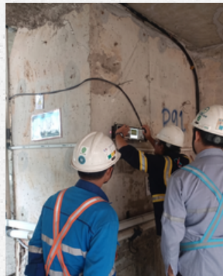
Project Ultrasonic Concrete Tomography (UCT) At Sawah Besar MRT D-WALL and Harmony Gambir – Central Jakarta
