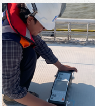
Project Ultrasonic Concrete Tomography (UCT) at Dock A – PT. Petrokimia Gresik
