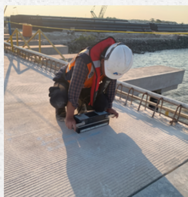
Project Ultrasonic Concrete Tomography (UCT) at Dock A – PT. Petrokimia Gresik
