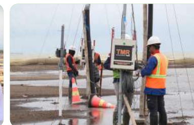
Strain Gauge Installation On Bamboo And Rope For Semarang – Demak Toll Road Construction
