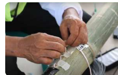
Strain Gauge Installation On Bamboo And Rope For Semarang – Demak Toll Road Construction
