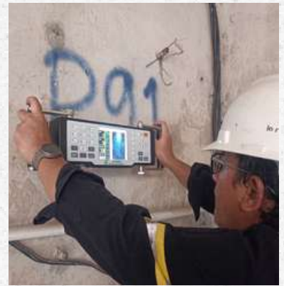
Project Ultrasonic Concrete Tomography (UCT) At Sawah Besar MRT D-WALL and Harmony Gambir – Central Jakarta
